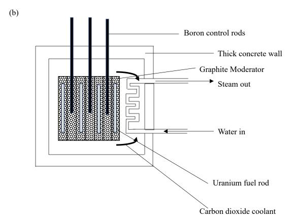
The atoms of uranium in the fuel rods capture a neutron and undergo a fission reaction producing barium, krypton, three neutrons and energy in form of heat according to the equation below
