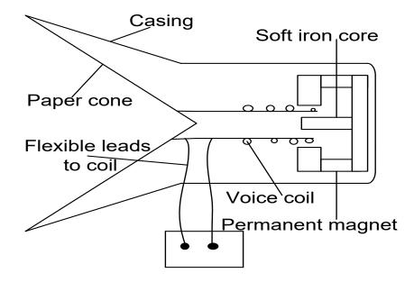
A varying electric current passes through the speech coils. The speech coils experience a varying force due to the magnetic field which causes them to move to and fro together with the paper cone attached to it. The paper cone sets the air into vibration causing the air to vibrate at the same frequency as the current flowing through the speech coils reproducing the original sound.
