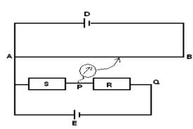
In the circuit shown above D is a driver cell of negligible internal resistance and e.m.f. 3V. AB is a uniform slide wire of resistance  $20\Omega$ . S is a standard resistor of  $5\Omega$ . E is a cell of e.m.f. 2.5V. R is an unknown resistor. When the galvanometer is connected at P the
