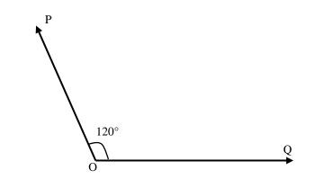
The force P has a magnitude 20N and Q has a magnitude of X newtons. The resultant of P and Q is 3X newtons. Find;
