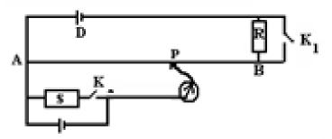
When both switches are open balance length is 20 cm. When only  $K_2$  is closed the balance length is 15 cm.
