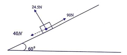
Three force of 90N, 40N and 24.5N act on a block placed on a smooth surface inclined at an cangle of 60° to the horizontal. Calculate
