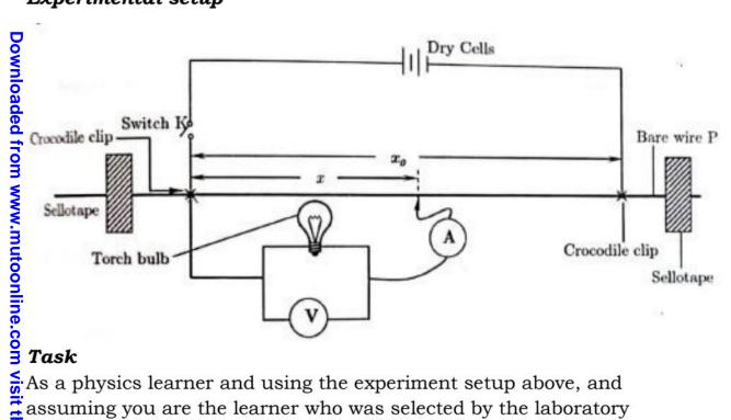
assuming you are the learner who was selected by the laboratory technician, carry out a scientific investigation to determine the resistance of the bulb filament of the simple bulb.
