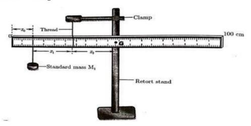
As a physics learner and using the arrangement of the apparatus above, carry out a scientific investigation to help the other learners determine the mass of the uniform metre rule they designed as their project work.
