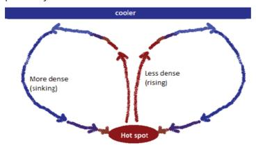
Fig. 6.7: Illustration of convection
