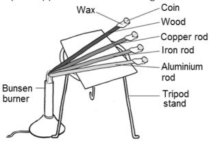
Fig. 6.5: Investigating rates of conduction
