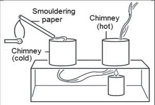
Fig. 6.10: Demonstrating convection in air
