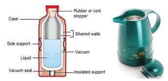
Fig. 6.20: Parts of a vacuum flask
