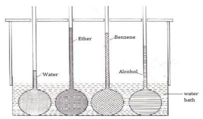
Fig. 7.6: Comparing liquid expansion
