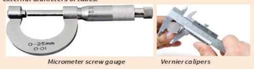
Fig. 2.4: Instruments for measuring small lengths
