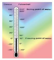
Fig. 5.1: Temperature scales
