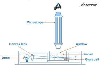
Fig. 3.8: Smoke cell experiment
