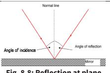
Fig. 8.8: Reflection at plane surfaces
