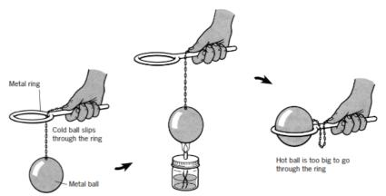
Fig. 7.1: Ball and ring experiment
