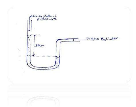
If the density of water is 1000kgm<sup>-3</sup> and H = 76cmHg. Calculate pressure in Nm<sup>-2</sup>.
