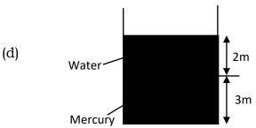
If the density of mercury is 13600kgm<sup>-3</sup> and the density of water being 1000kgm<sup>-3</sup>. Calculate the pressure exerted at point A.
