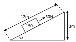
A load of 150N is raised on an inclined plane through a distance of 3m by an effort through 50N that moves а distance of 12m. Calculate (iii) Efficiency.
