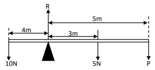
A uniform metre rule is pivoted at 20cm mark as shown. Find the weight of meter rule.
