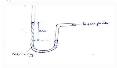
Find the gas pressure if the atmospheric pressure H = 76 cmHg and density of mercury  $13600 \text{kgm}^{-3}$
