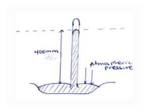
Calculate the atmospheric pressure
