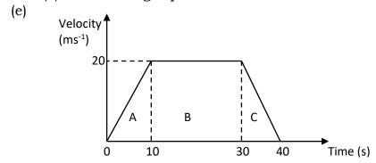
The diagram above represents a velocity – time graph for the motion of the body. Calculate;
