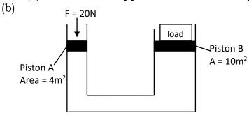
Calculate the weight of the load.
