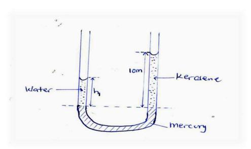
If the density of water is  $1000 kgm^{\text{-}3}$  and density of kerosene being  $800 kgm^{\text{-}3},$  calculate the height  $h_1$
